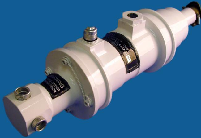
S-76 Rotor Brake Accumulator
